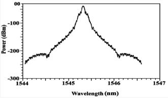
Figure 1.19 Wave length of delay-and-add operation at specplt\_8 scope in duobinary transmission system
