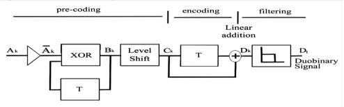
Figure 1.5 Basic structure of a duobinary encoder
