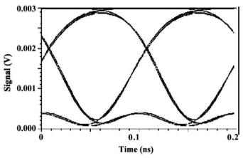
Figure 1.14 Eye diagram of duobinary filter at receiver-2 scope in duobinary transmission system
