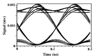
Figure 1.12 Eye diagram of duobinary Filter at receiver-1 scope in duobinary transmission system
