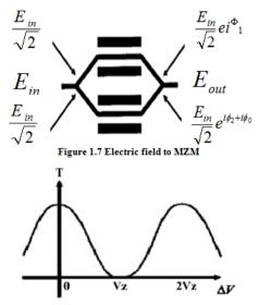
Figure 1.8 Electrodes voltage different to the MZM
