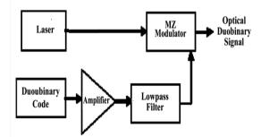
Figure 1.4 Block diagram of generating optical duobinary signal
