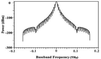
Figure 1.17 Frequency oscillation of base band signal of delay-and-add circuit in duobinary transmission system
