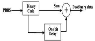
Figure 1.3 Block diagram of converting duobinary code from binary
