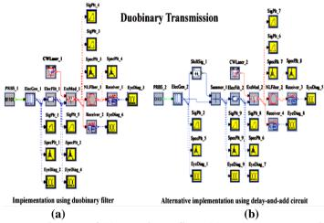
Figure 1.11 Simulated block diagram of (a) Duobinary filter (b) Delay -and –add circuit in duobinary transmission in fiber optic communication using Optsim software
