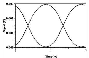
Figure 1.15 Eye diagram of delay-and-add Operation at receiver-2 scope in duobinary transmission system
