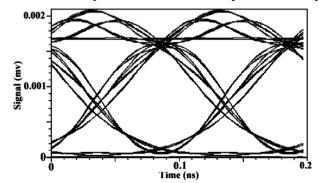
Figure 1.13 Eye diagram of delay-and-add operation at receiver-3 scope in duobinary transmission
