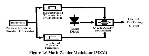
Modulator splits an incoming light signal into two waveguide branches. The two branches experience different optical delays, depending on the voltage applied to each arm, and then recombine constructively or destructively.
